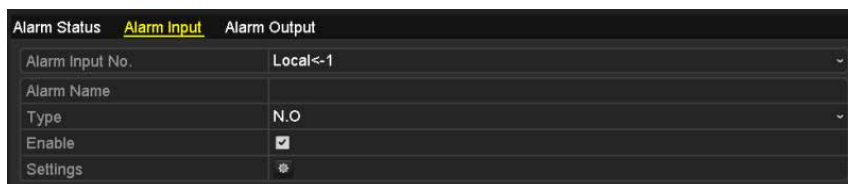
Figure 5. 15 Alarm Settings- Alarm Input
